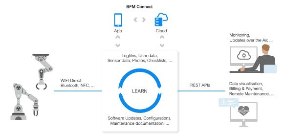
Integrate non-networked machines into the smart service world with BFM Connect
